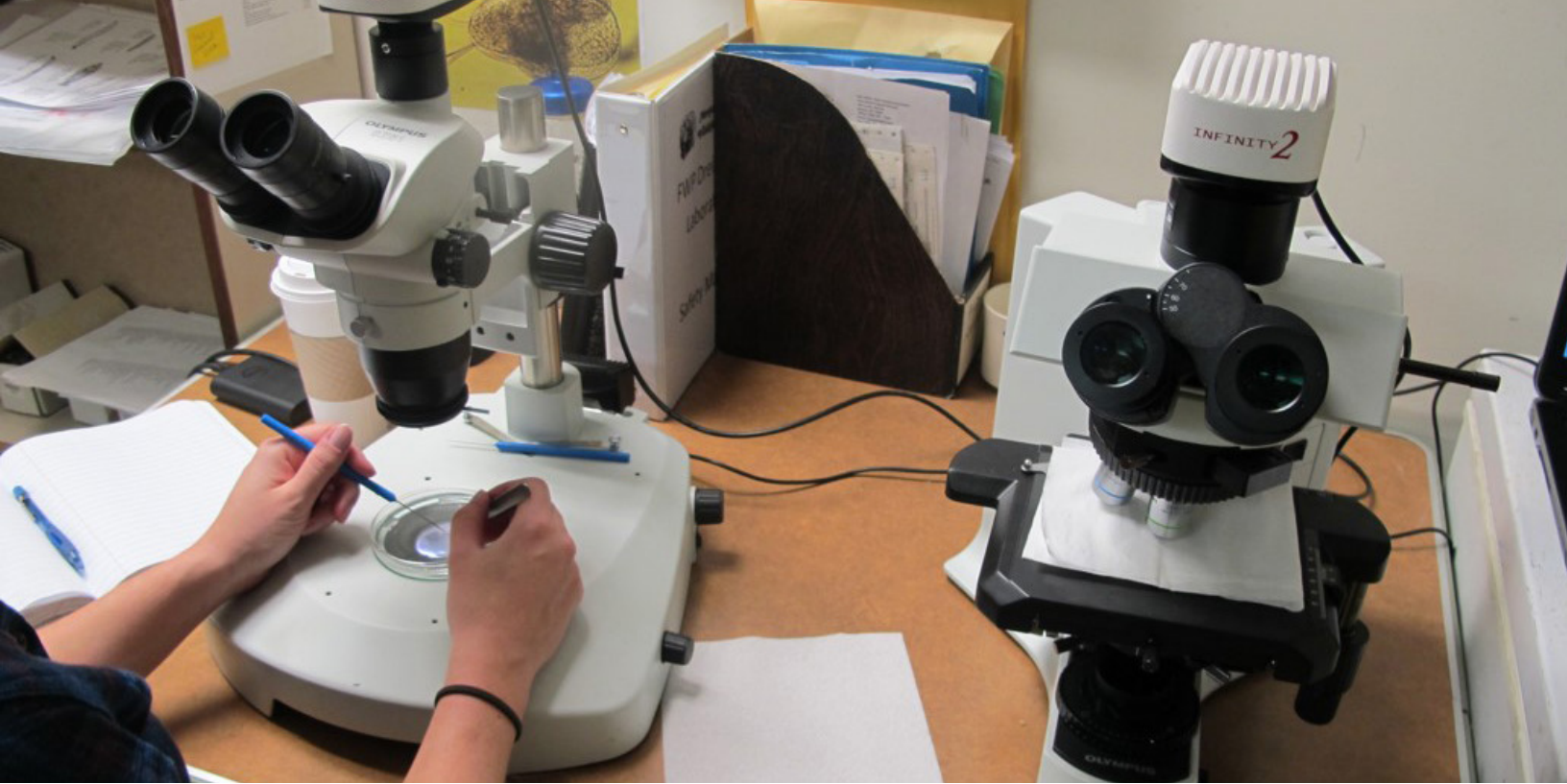
Plankton samples are examined under a microscope for dreissenid veligers (microscopic larvae)
